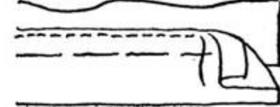
Lapped or tucked seam
